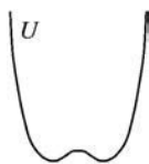
Fig. 5.4 Shape of potential energy between atoms is modified to wine-bottle-like when the interatomic distance is increased.
